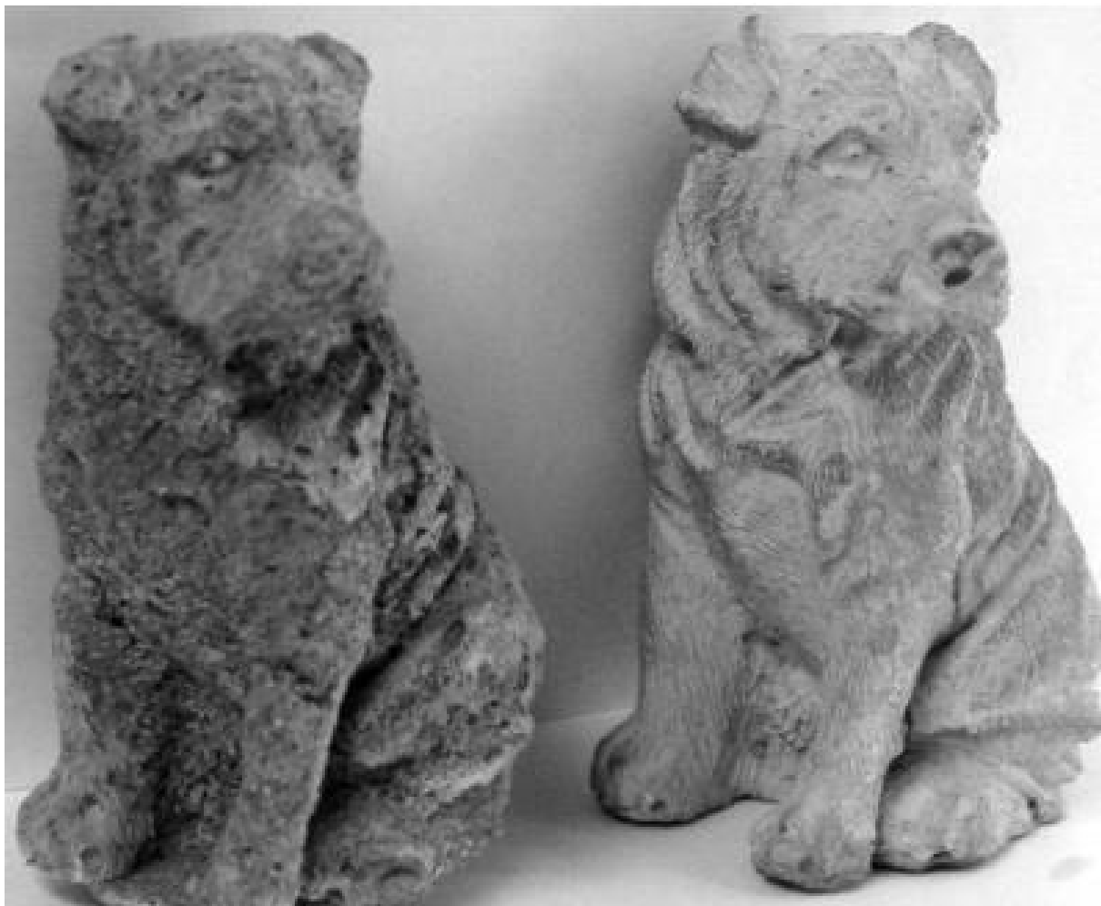
Figure 10: sculptures made by conventional OPC (left) and by refined HPPC (right).
