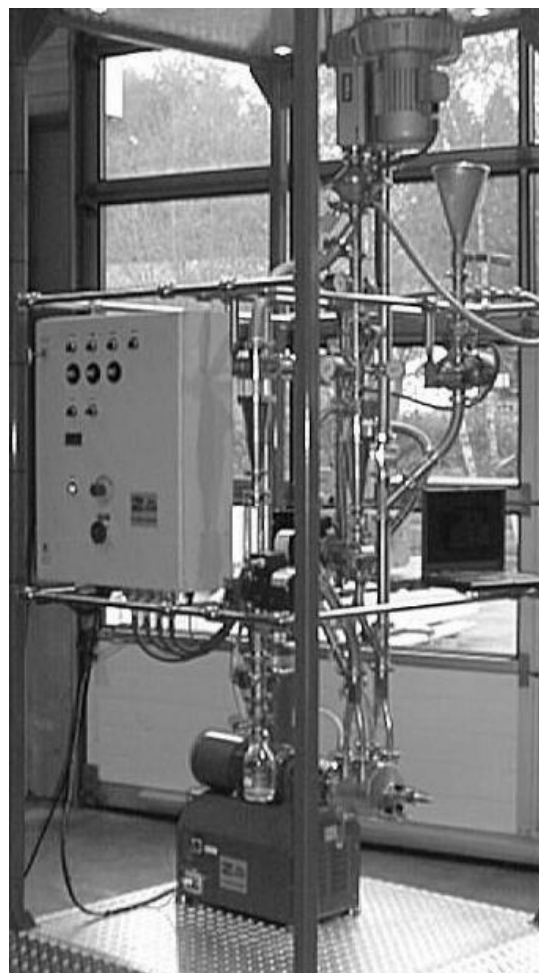
Figure 19: VS01a (Simoloyer CM01-2sl) pilot plant in compression mode, picture: Zoz, Germany)
