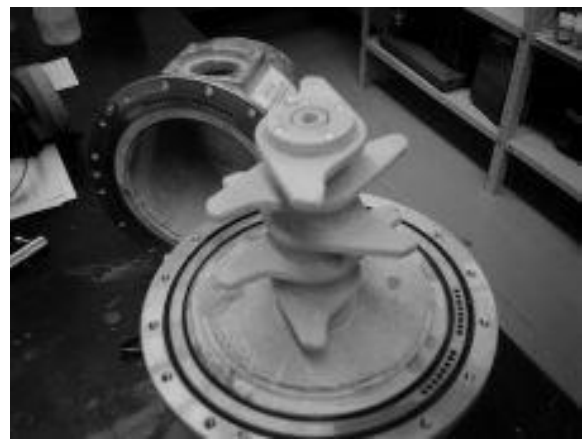
Figure 16: no damage on the rotor-blades, wear surprisingly low, diameter loss less than 2 mm (after 4000 h !)
