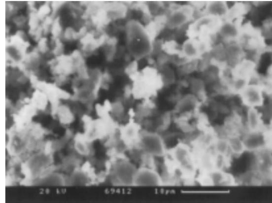
*Fig. 15b: Particle sizes of  $\text{Al}_2\text{O}_3\text{-SiC}$  powder after processing (SEM-backscatter electron)*
