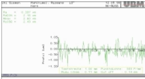
Fig. 11a: Roughness measurement of a new ball
