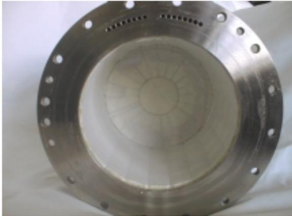
Fig. 5: Grinding chamber lined with  $\text{Al}_2\text{O}_3$  after 5h: Hardly wear of the  $\text{Al}_2\text{O}_3$  lining could be observed
