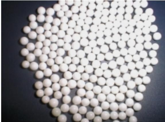
*Fig. 13a: New yttria stabilized ZrO<sub>2</sub> balls (Nagase & Co., LTD, Japan)*
