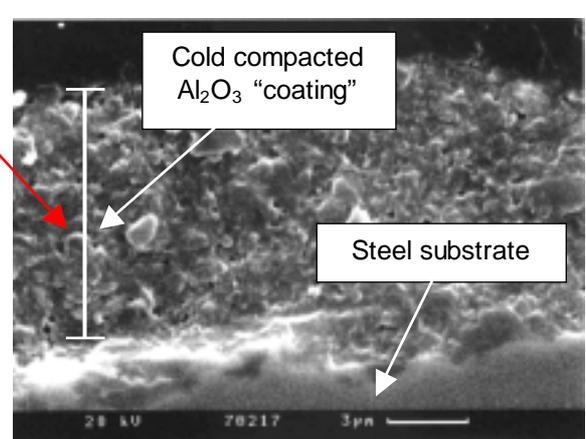
Fig. 10b: Cross section of a ball with cold compacted “coated”  $Al_2O_3$  layer after
