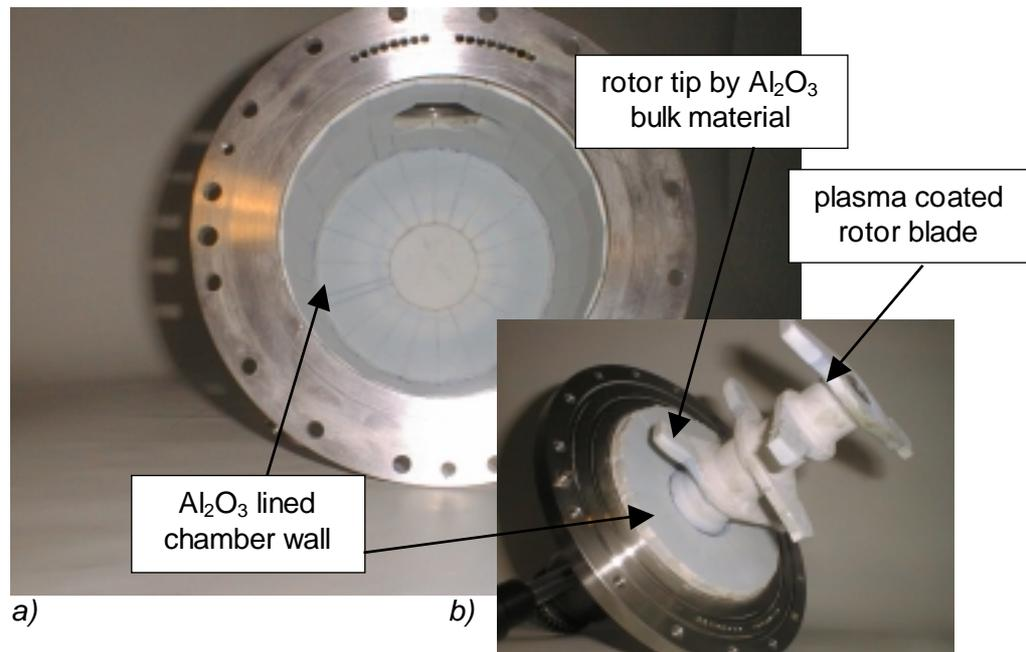
Fig. 2: Grinding parts of prototype 1. a) chamber with  $\text{Al}_2\text{O}_3$  lining; b) rotor with  $\text{Al}_2\text{O}_3$  full material rotor tips and plasma coated rotor blades
