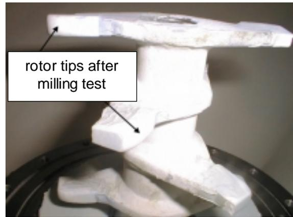
Fig. 6:  $\text{Al}_2\text{O}_3$  rotor after 3h milling
