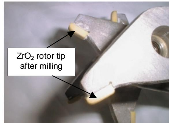
Fig. 9b: ZrO<sub>2</sub> rotor after 1h milling
