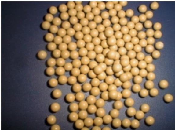
Fig. 12a: New ZrO<sub>2</sub> balls
