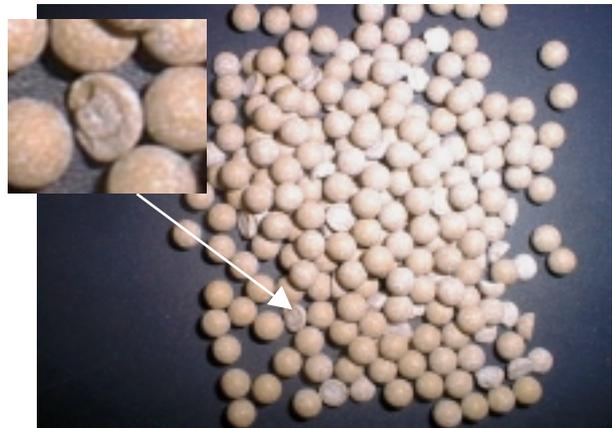
Fig. 12b: ZrO<sub>2</sub> balls after 1 h milling
