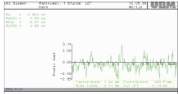
Fig. 11b: Roughness measurement after 14h
