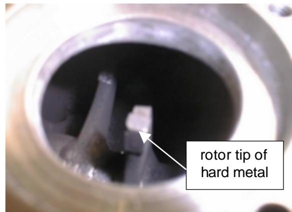
Fig. 8: Hard metal rotor after 20h:
