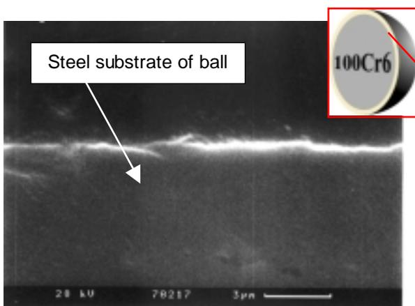
Fig. 10a: cross section of a steel ball before milling
