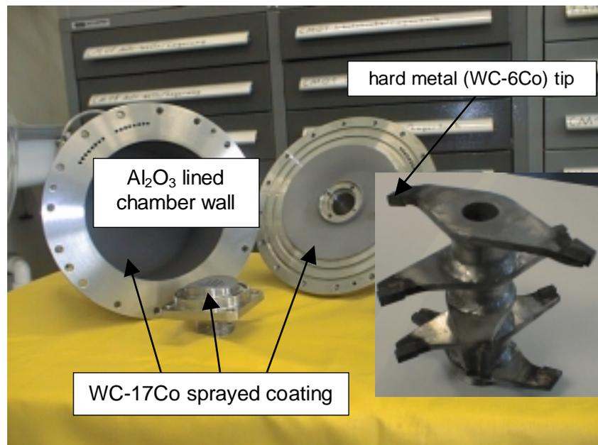
Fig. 3: Grinding parts of prototype 2, WC-17Co coated chamber
