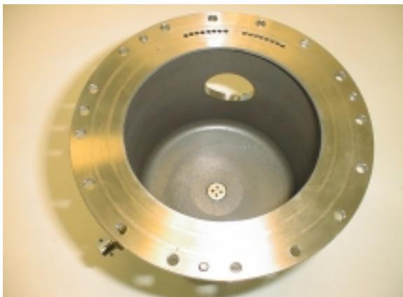
Fig. 7:  $\text{WC}+17\text{Co}$  coated milling chamber after 3h test: The  $\text{WC}+17\text{Co}$  thermal spray coating remains
