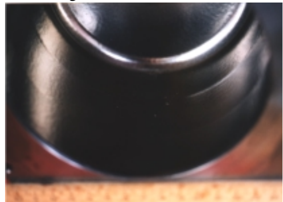
Figure 10b: grinding chamber after cycle operation
