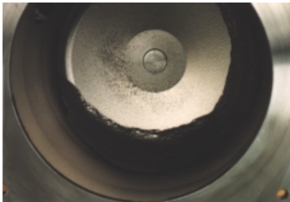
Figure 10a grinding chamber after constant operation
