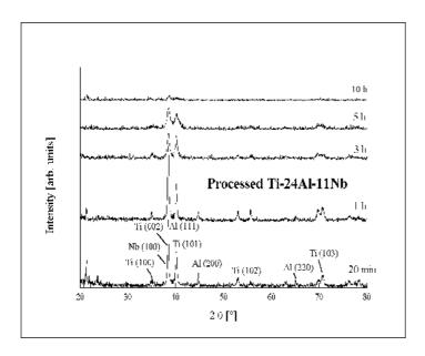
A phase transformation into an fcc crystal structure can be assumed by the above X-ray diffraction patterns between 10 and 15 hours as found by *Suryanarayana et al.* for Ti-33Al. After 15 hours of mechanical alloying any reflexes are absent.
