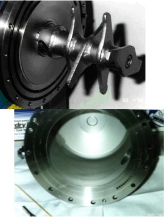
Fig. 11.a+b: Grinding chamber after cycle operation (Fe<sub>3</sub> Al, Oak Ridge National Laboratory, Oak Ridge, TN)
