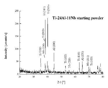
Fig. 2: X-ray diffraction pattern of the starting powder blend
