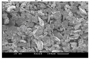
Fig. 7.a: Processed powder after 10 h using cycle operation
