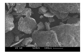
Fig. 4.b: Processed powder after 1 h
