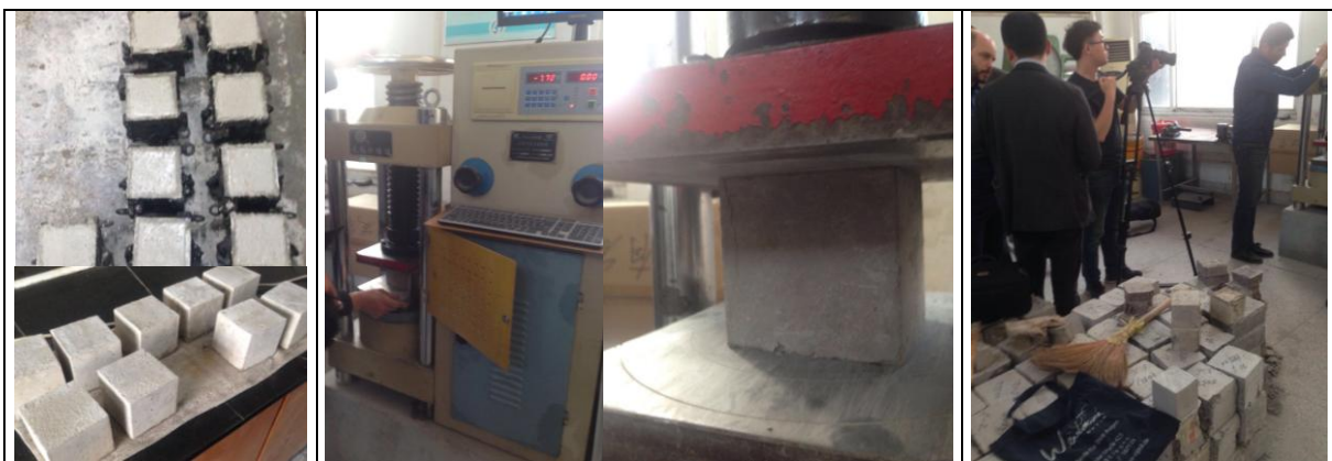
f.l.t.r.: standard test cubes before and after encasing, test apparatus in Changzhou, video documentation of test series
