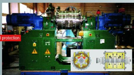
Production unit with a 100 liter chamber. The cross sections through the grinding chamber visualize the working principle. The rotor is the tool to transfer the kinetic energy into the grinding media and these transfer further into the powder materials.
