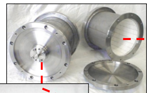
Steel container with lining Al_2O_3 RBA02 & RBA05
