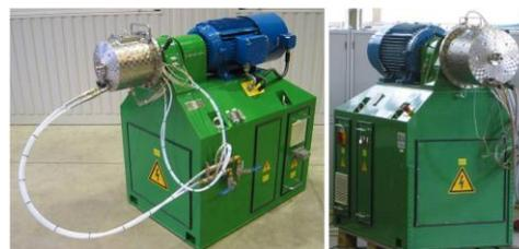
Figure 3. Simoloyer<sup>®</sup> CM08-8lm (left) and CM20-20lm high energy ball mill (right).
