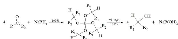
Fig. 1. Solid state reduction of carbonyls with NaBH<sub>4</sub>.
