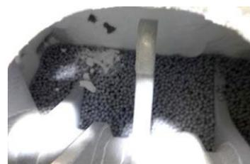
Fig. 6. Holdup in the grinding unit after neutralization.
