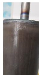
Top of capsule - gas tight welded
